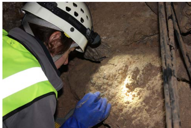
Figure 5. Lila Jones using a dental pick to loosen embedded sediments. William Tucker
