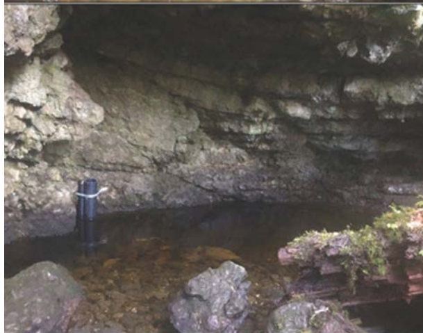
Figure 4: Stilling wells at the following study sites: (a) Zina Cave baseflow, (b) Walkabout Cave insurgence, (c) Walkabout Cave resurgence.
