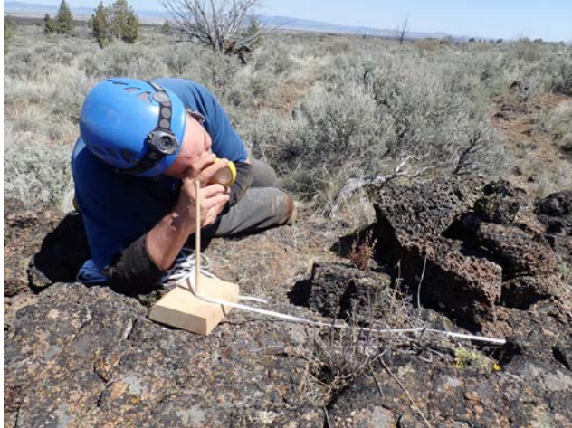
Paul McMullen uses a standoff to reduce magnetic interference with the compass. Mark Jones
