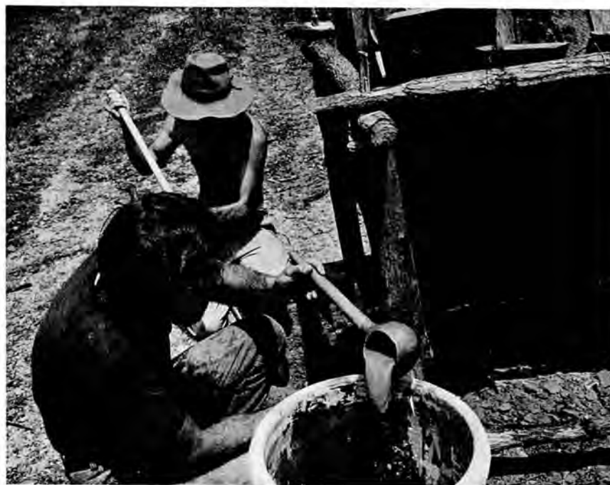
Figure 18. (a) Removing liquor from saltpetre vat. (b) An authentic 1812 vintage Mammoth Cave boiling kettle, near Brownsville, Ky.
