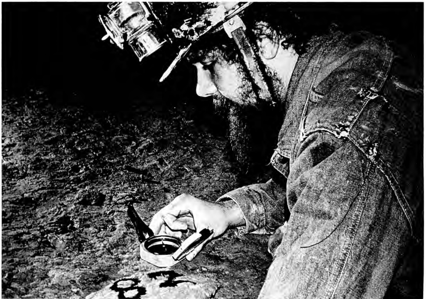
Figure 2. Richard Zopf uses a Brunton compass to measure bearing between survey stations in the Flint-Mammoth Cave System. Photo by Roger Brucker
