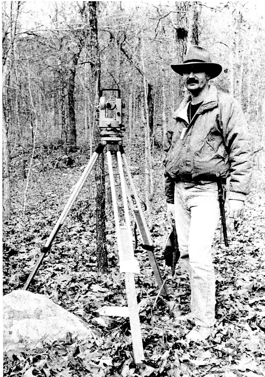
Figure 2: Mike Pearson waits for the range pole to be placed while running a transit survey near Fitton Cave, Arkansas ( Photo by Pete Lindsley ).
