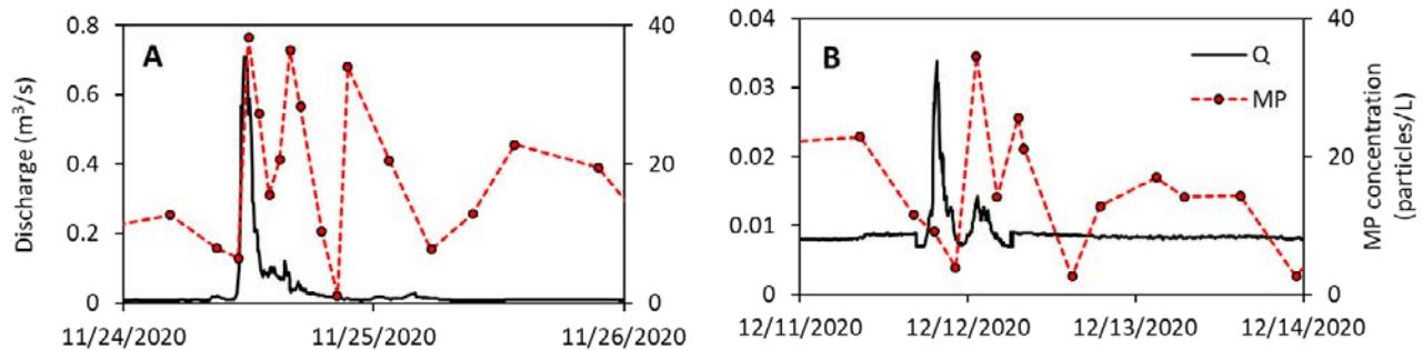
Fig. 5. Discharge (Q) and microplastic (MP) concentration during floods sampled in November 2020 (A) and December 2020 (B).
