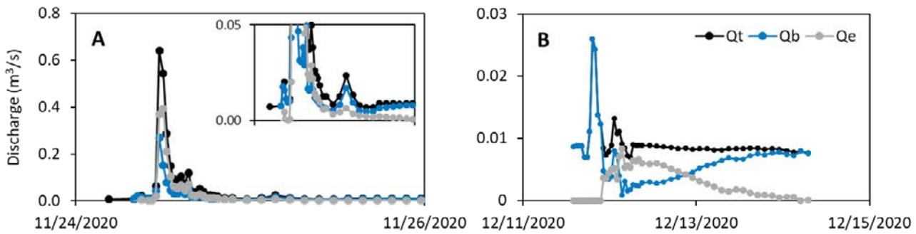
Fig. 4. Flood hydrograph separations performed using  $\delta^2\text{H}$  data. The hydrograph separations show the timing of the baseflow ( $Q_b$ ) and event water ( $Q_e$ ) components of the total discharge ( $Q_t$ ) for the November 2020 (A) and December 2020 (B) floods.
